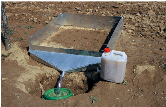
Fig. 2. Erosion plot on bare land in an olive grove with collected weekly runoff and eroded material (7 April 2005–14 April 2005; photo: Matija Zorn)
