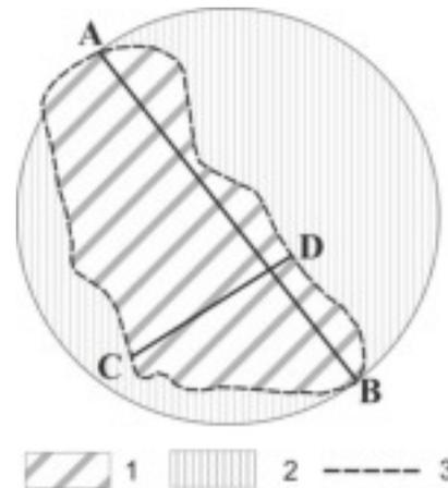
Fig. 2. The parameters computed for micro-depressions (AB – major axis ( $L$ ), CD – minor axis ( $W$ ), 1 – micro-depression area ( $Ad$ ), 2 – area of the circle having the same diameter as the depression's major axis ( $Ac$ ), 3 – perimeter of the micro-depression ( $Pd$ ).
